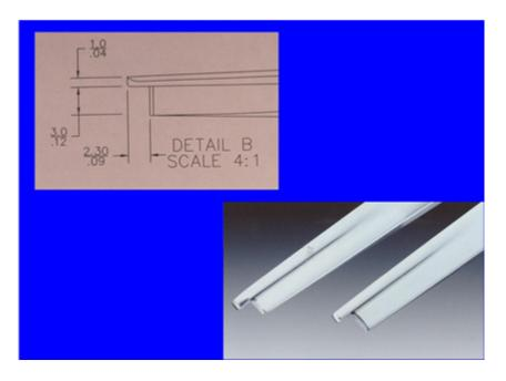
So as I mentioned, we worked with an instrument company to design 2.5 and 3-mm osteotomes with a little guard. That little guard is just so that you can engage the bone and so the osteotome won't slip off, so it makes it a very reliable instrument and a reliable
